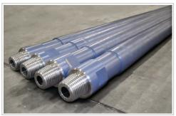
Mincon rotary drill pipe is manufactured to customer requirements for outside diameter (O.D.), wall thickness, length, and specific drill rig wrenching configurations. Tool joints are precision machined from premium quality materials and then reinforced with ultra-hard materials to withstand premature wear from the most abrasive rock and drilling conditions.
