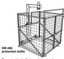
The protection trellis is used to secure loose loads handled with pallet forks KM 415 and KM414 – e.g. brick packages, loose construction materials. When handling loose material, a protection trellis or net to secure the load, is obligatory (EN 13155). The maximum capacity is 2000 kg. The protection trellis can be mounted within a few minutes and is thus suitable for each construction site without any problems.
